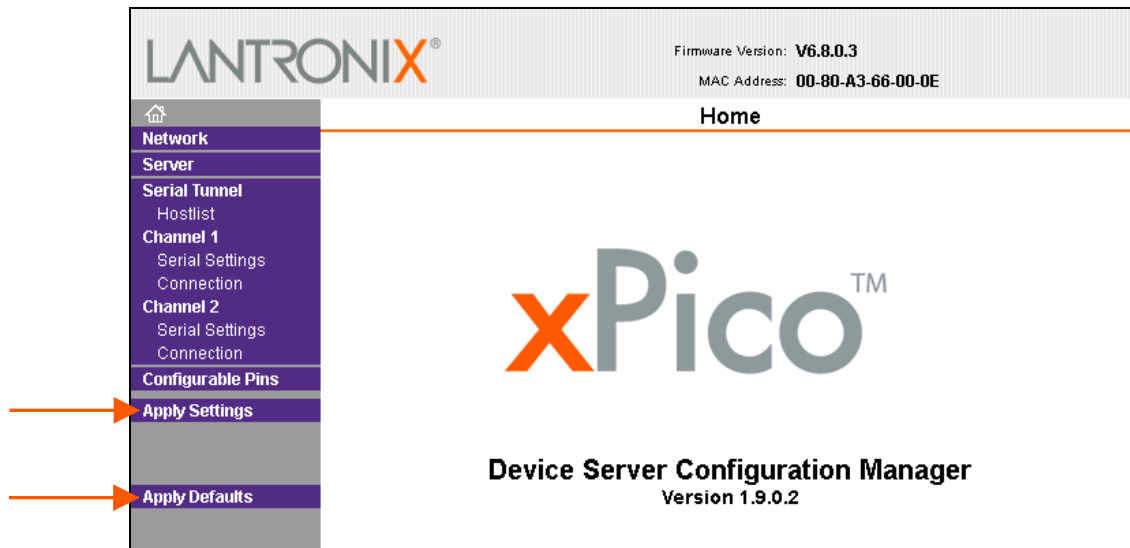
Figure 4-10. Apply Settings and Apply Defaults
